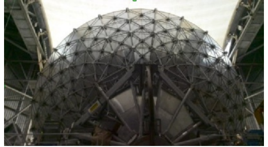
15 m of JCMT: The 15 m primary mirror of the JCMT taking data through its protective membrane during daylight.
